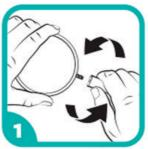
**Pole assembly**Attach the metal ring to the telescopic pole by rotating it.
